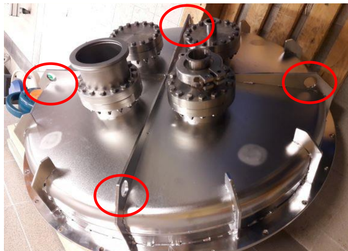
Figure 8 the four CB interfaces (eyelets) are shown. Only two of them shall be used
