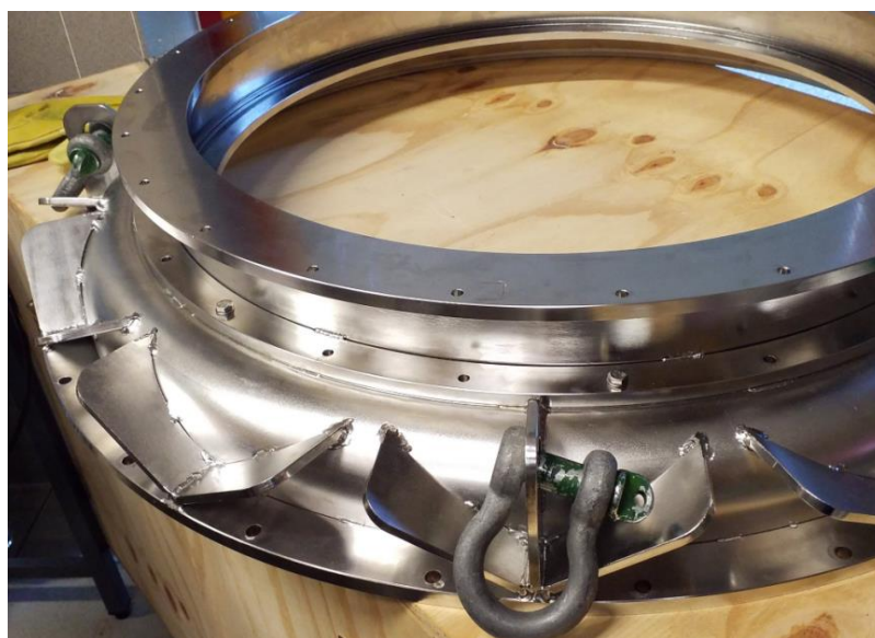
Figure 11 Top flange detail: the vacuum window is dismantled. The two eyebolts to lift the flange are visible.
