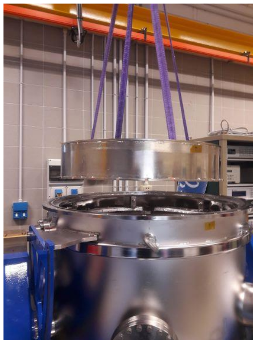
Figure 14 The IR filters holder hanging by the two belts on the CB hanger.
