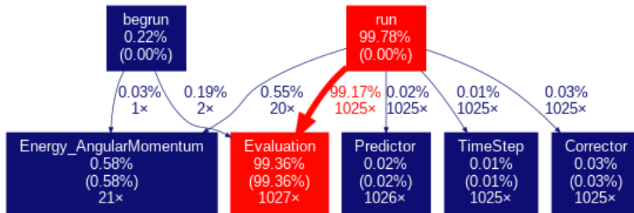
Figure 1: Call graph of EXAHIGPUS profiled using gprof tool. The figure shows nodes and edges above the threshold 0.01.
