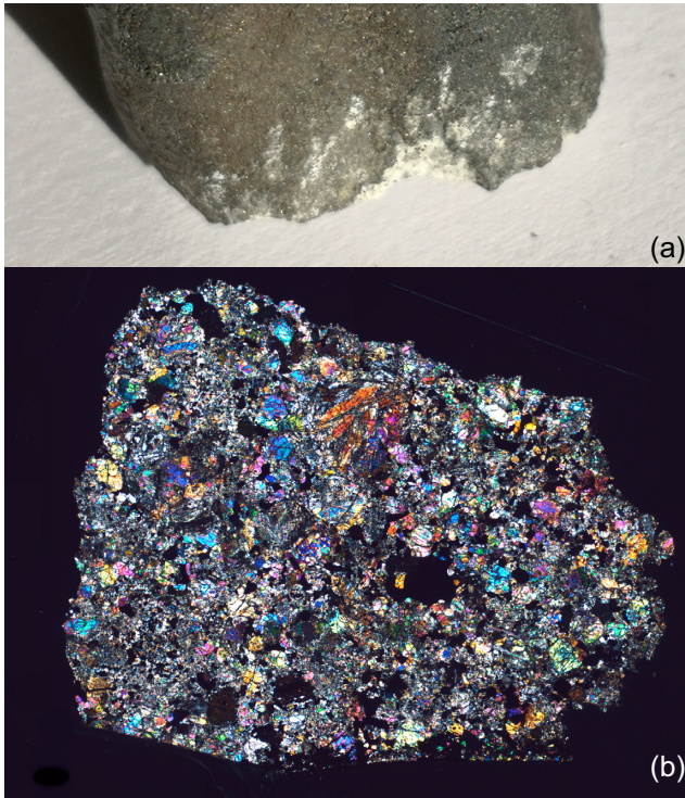
Figure 2. Details of the larger fragment F2 of the Cavezzo meteorite. (a) White streaks occur on one edge of F2, suggesting on-ground breakup of the original body; (b) photomosaic of polarizing optical microscope images (transmitted light, crossed polars) of a thin sections obtained from F2 (field width 12 mm) showing chondrules and chondrule fragments distributed in the matrix.
