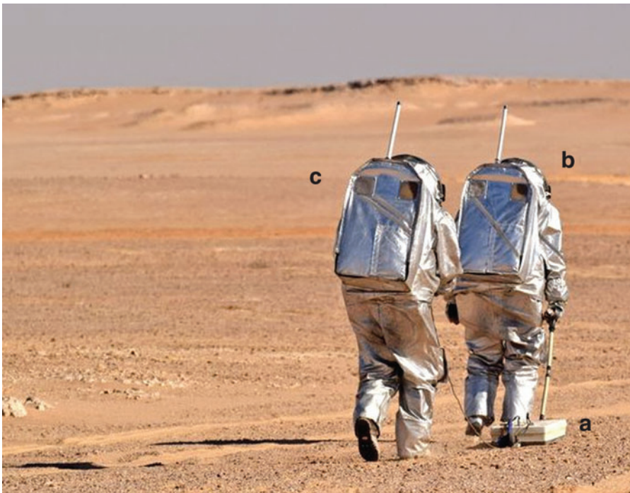
FIG. 4. ScanMars operations during an Extra Vehicular Activity (EVA). The radar antenna sled ( a ) is being pulled along the planned transect by astronaut ( b ), while a second one ( c ) carries the Central Processing Unit (CPU) which displays a live view of the data being acquired along with the operative parameters of the instrument (picture credits OeWF). Color images are available online.
