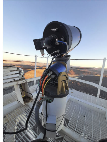
Figure 2. ESO MASS-DIMM located at Cerro Paranal, site of the VLT in Chile. The instrument is placed on top of a 7-m high tower. Credit: Angel Otarola, ESO.
