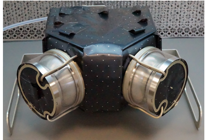
Fig. 4. Flight model of the SWA-EAS unit, showing the two orthogonally-mounted cylindrical electron optics subsystems attached to the control electronics box (which is housed beneath the black multi-layer insulation (MLI) blankets). The curved aperture deflector plates, lying either side of the apertures themselves, can be seen through the entrance grid on both heads.
