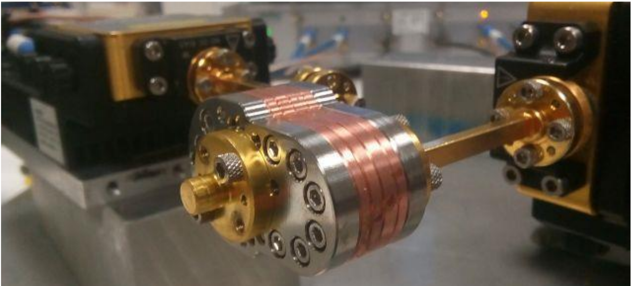
Figure 4. The new INAF OMT in CuTe under test at INAF/OAA
