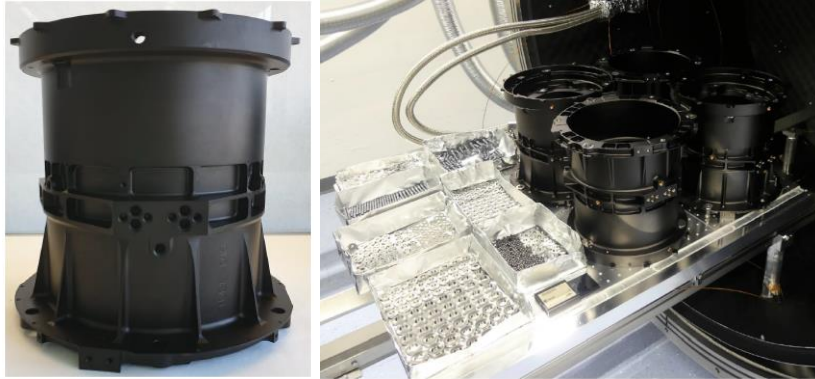
Figure 1. Tubes delivered by UBE. Left image shows the TOU Structure Tube after coating and the right image some of the Tubes after bake-out at UBE.
