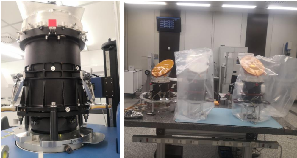
Figure 3. The PFM TOU during AIV at the Leonardo Company in the left. Serial production @ Leonardo Company in the right.
