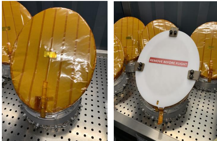
Figure 10. BA during the final cleaning phase under ISO5 tent. On the left, a detail of the red-tag soft cover is visible. On the right the red-tag hard cover is visible.
