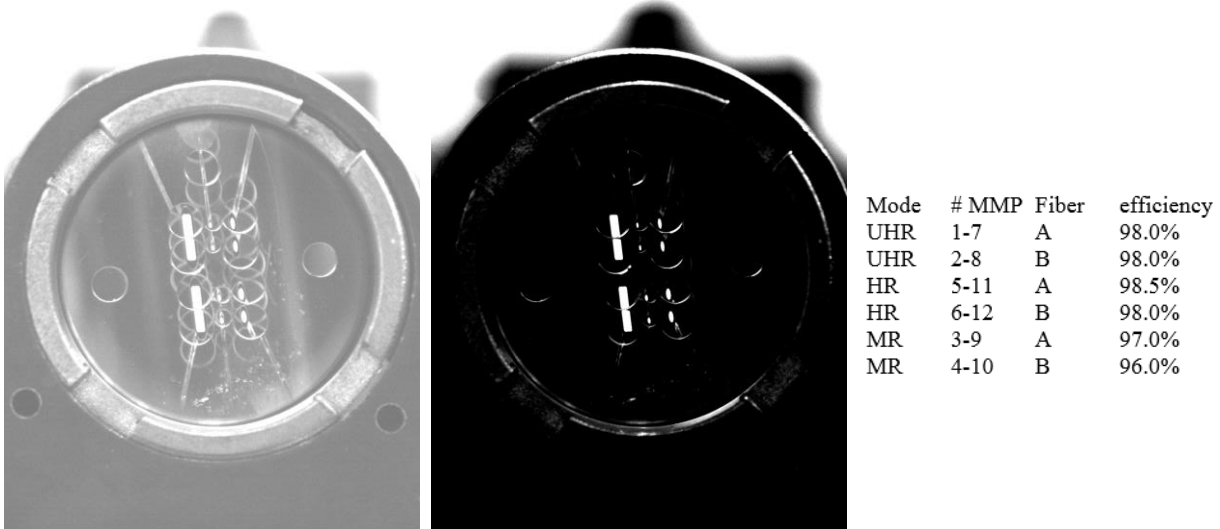
Figure 8: MMP#3 during integration in the APSU. Enhanced brightness image to show the mechanical references in the mounting (left); virtual slits on the MMP plane: four images for each observation mode, made by star and sky fibers, sliced in two (center); transmission efficiency of the single fibers (right).
