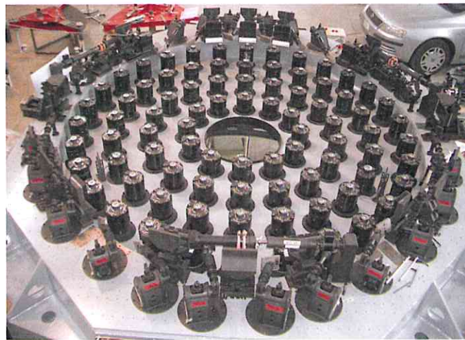
Fig. 2 – The axial and lateral supports before the installation of the mirror (top view).
