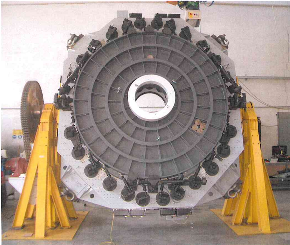
Fig. 15 – The mirror cell during tests on a motorized tilting device at Tomelleri s.r.l. premises.
