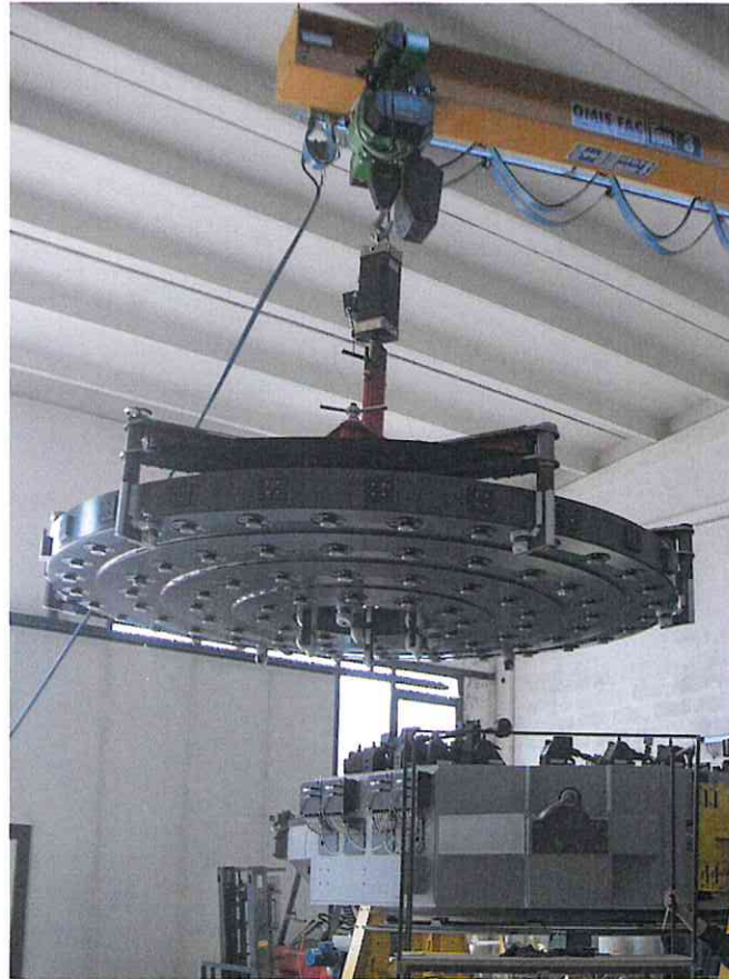
Fig. 11 – Primary mirror handling procedure (1/4): the mirror is lifted by its handling device, connected to a load positioner and the crane.
