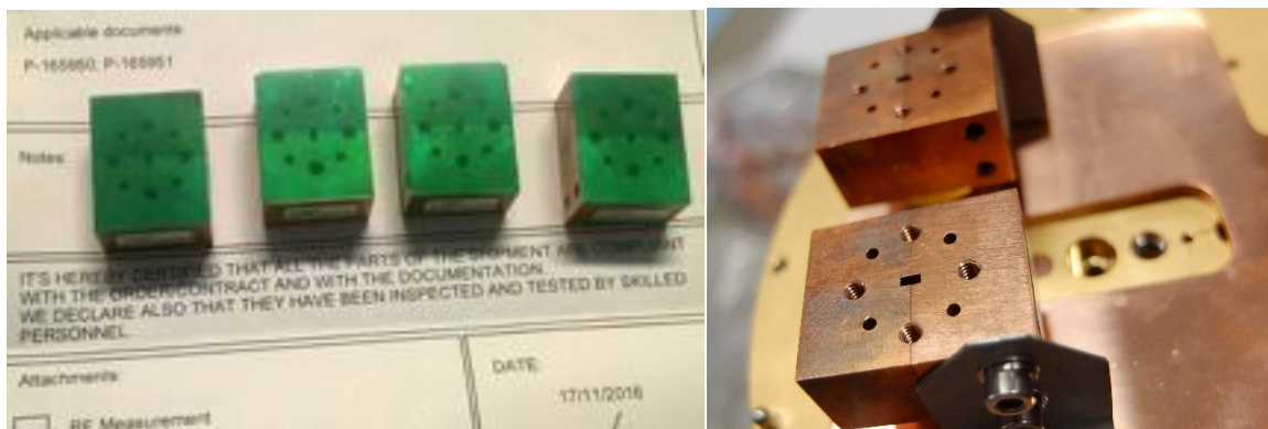
Figure 4. WR10-WR15 Transitions as arrived at INAF (left) and as mounted on the cartridge (right).
