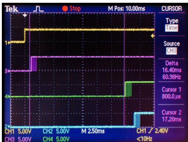
Figure 5: Shutter open signals jitter and timings.
