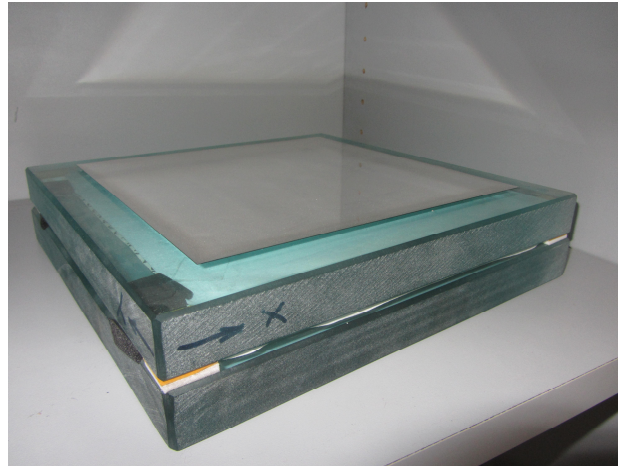
Figure 1 – first attempts of cold slumping of flat foils of glass (2005): the thickness of the foils was from 0.125 mm to 0.4 mm
