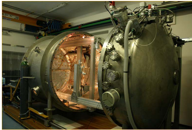
Fig. 11. The large Ion Beam Figuring facility operated at the Brera Astronomical Observatory – INAF.
