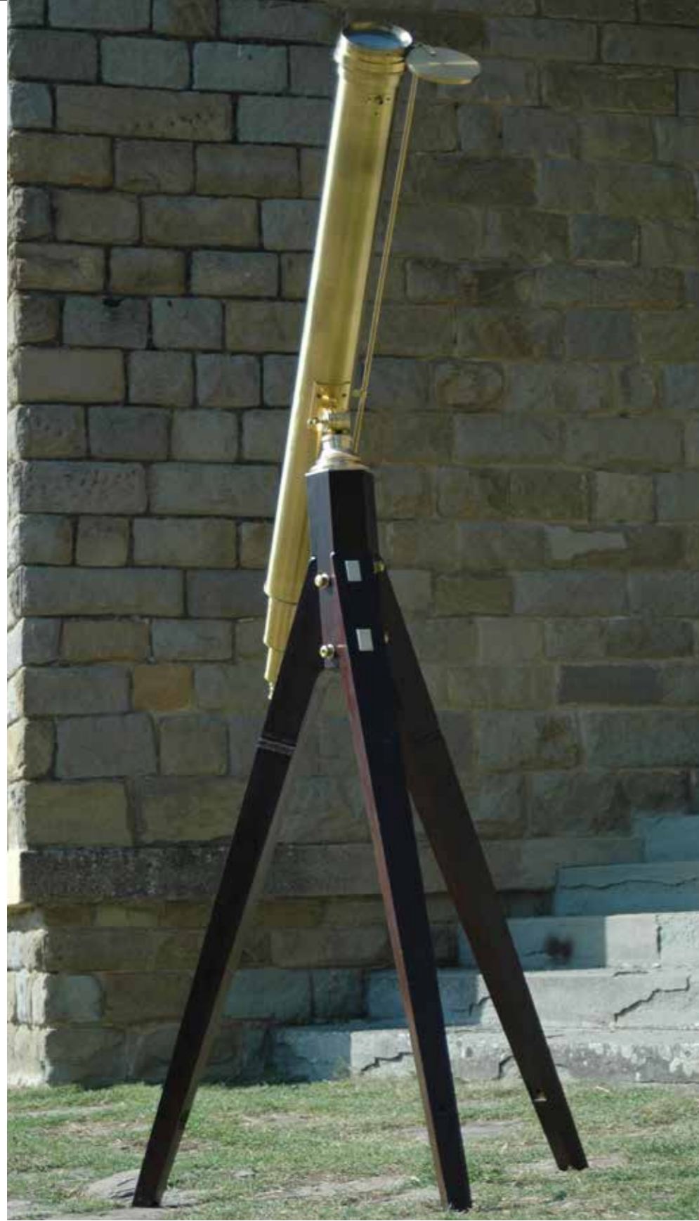
FI. 09. REFRACTING TELESCOPE Steinheil (objective), Munich 1858 brass, wood, glass (objective: 108 mm diameter, 1620 mm focal distance) INAF-Arcetri Astrophysical Observatory, inv. Coll. Scient. e Museali n. 107005001
