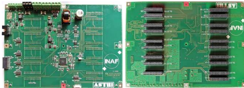
Figure 3. mainboard PCB (dimensions 210mm x 150mm). In the centre of the board the NXP Kinetis microcontroller is placed, which manages the communications with the BEE, the daughterboards and the other mainboard. The picture on the right side shows the layer where the connectors are placed for the daughterboards insertion.
