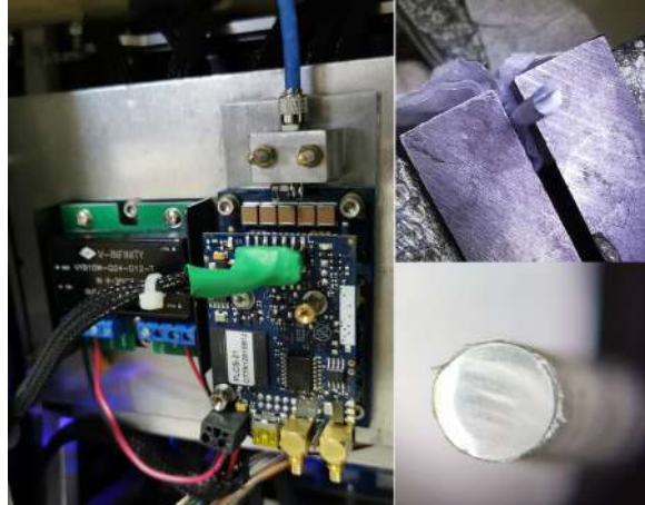
Figure 12. The Picolas driver on board of the ASTRI-Horn camera. The aluminum block couples the laser with the fiber and allows the heat dissipation of the diode to the metal plate. On the right the figure shows the finishing of the optical fiber input after the lapping process.
