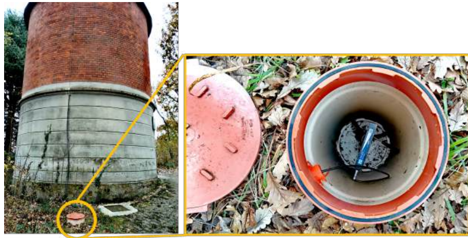
Figure 2. Left: The "Marcon" dome with the magnetometer shaft. Right: The magnetometer inside the shaft and installed on the tripod.
