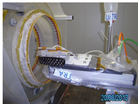
Fig. 12 The polishing phase with a pitch tool. The shell is mounted on the lathe with the optical axis in horizontal position. A liner carriage drives the oscillations of the pitch tool along the optical axis. \text{CeO}_2 slurry is distributed.
