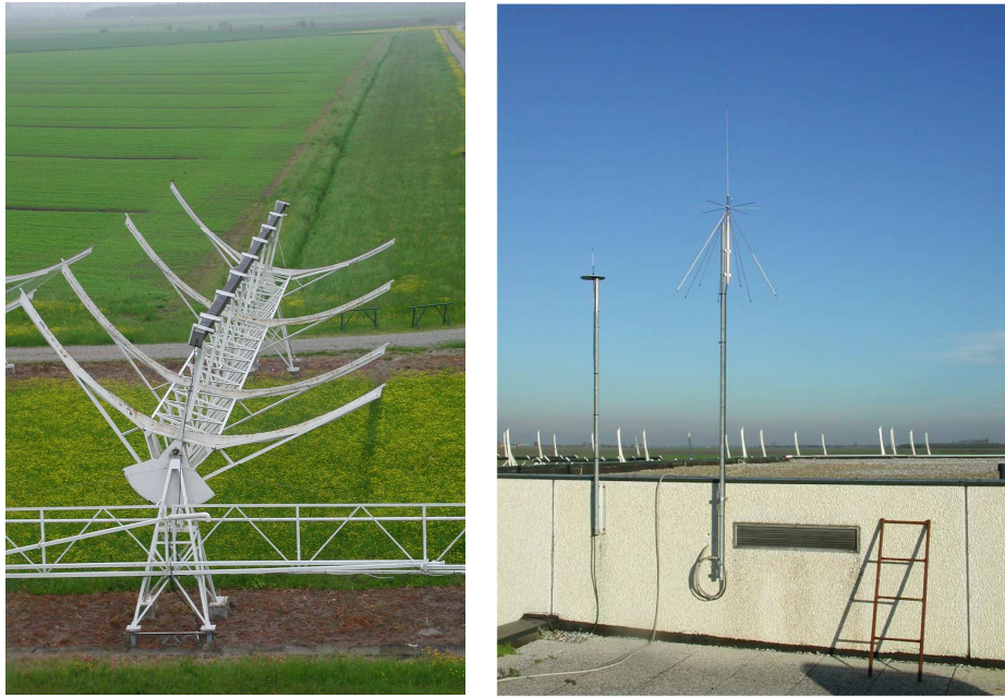
Figure 6.7: A channel of the Medicina Northern Cross array used as primary channel (left side) and a broadband omni-directional antenna used as auxiliary channel (right side).
