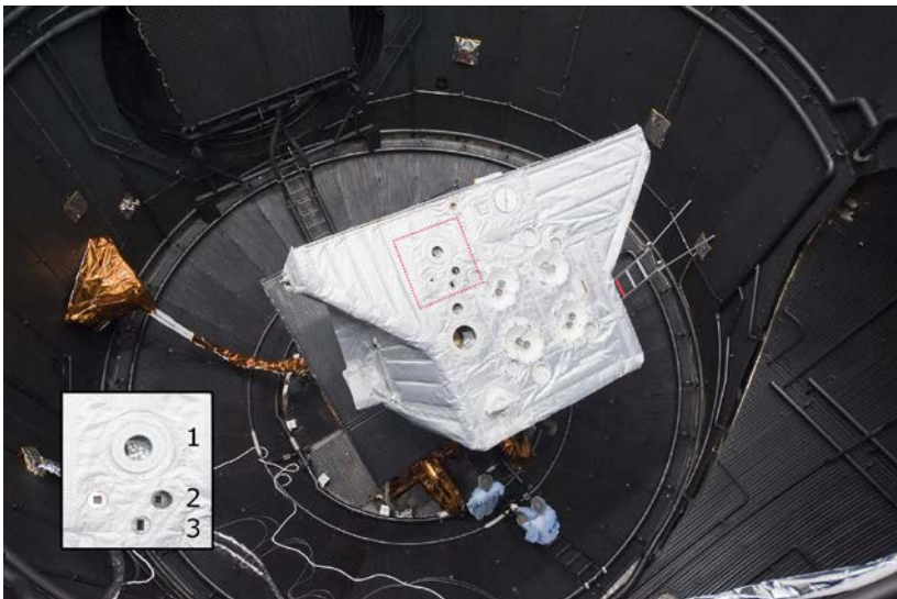
Figure 1.6. BepiColombo MPO Structural and Thermal Model (STM) inside the Large Space Simulator (LSS) at ESTEC Test Centre (courtesy of ESA). The red square indicates the location of SIMBIOSYS suite, also shown in the inset: 1) HRIC; 2) STC (both central holes); 3) VIHI.
