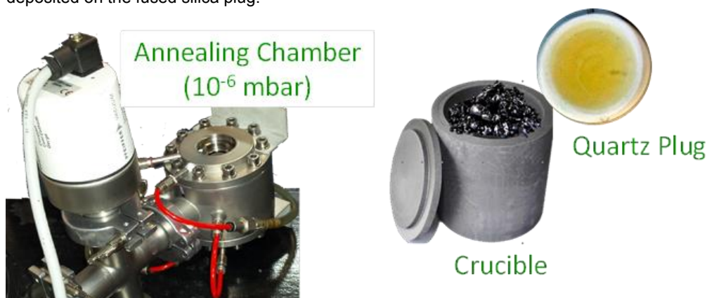
Figure 1: Experimental set-up: the high-vacuum annealing chamber for the thermal treatment (left) and the crucible with the fused silica plug (right).
