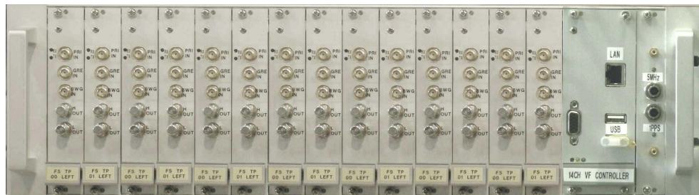
Fig. 8. Photo of the total power backend.
