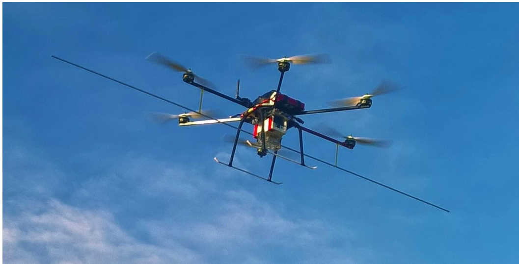
Figure 2. The flying artificial test source consisting in the UAV equipped with the RF transmitter and the 2-m long dipole antenna.
