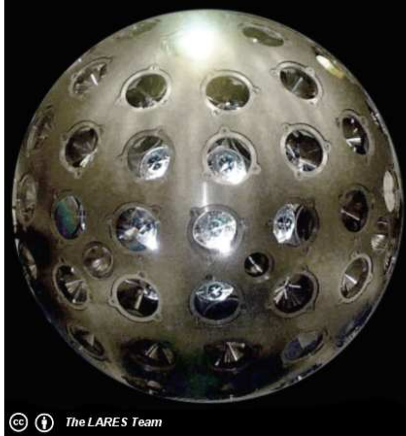
Figure 2. Picture of the LARES satellite (credits from LARES Mission: CC BY 3.0; see also www.lares-mission.com/gallery.html ). LARES is made of a unique piece of tungsten (THA-18N, composition 95% of W and 5% of Cu and Ni) and its surface is covered with 92 CCRs for SLR tracking. The CCRs mounting system is quite similar to that of the two LAGEOS, the most important difference is that the mounting rings and the screws are made of the same tungsten alloy of the satellite. The satellite radius is 18.2 cm and its mass is about 386.8 kg. The satellite orbit is almost circular with a semi-major axis of about 7820 km (corresponding to an orbital period of about 6883 s). LARES has been launched with the qualification flight of the new European launcher VEGA.
