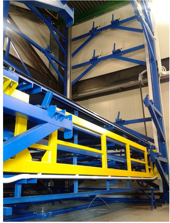
Fig. 2. Mechanical structure of the detector prototype. Four XY detection planes ( 18\text{ m}^2 each) are to be installed on this structure, with a relative distance of about 7 m between the top and bottom planes.
