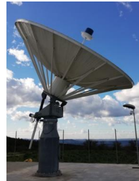
Fig. 2 BIRALES transmitting antenna (TRF).
