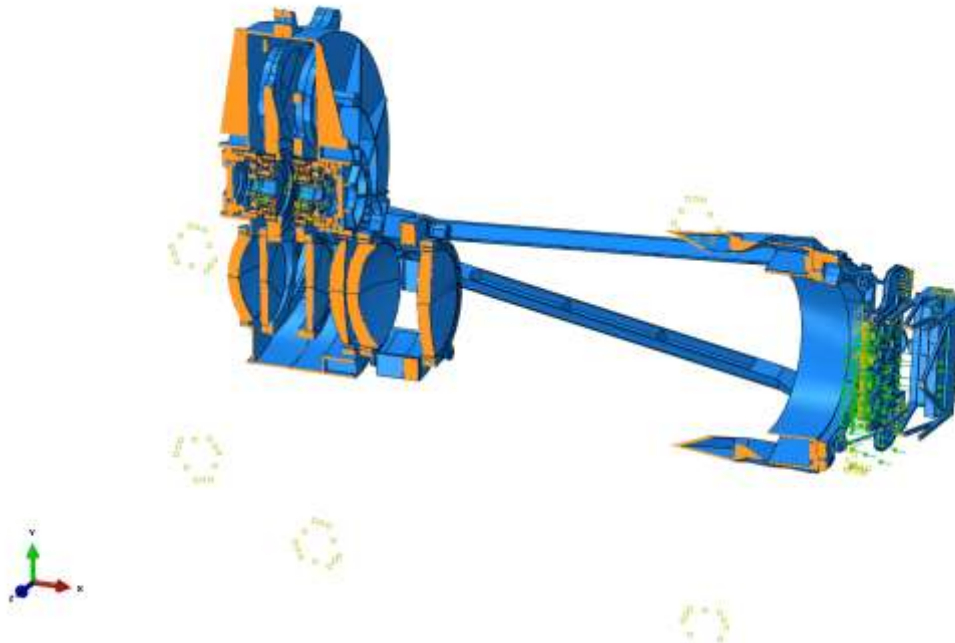
Figure 9-5 All loads applied on steady state analysis
