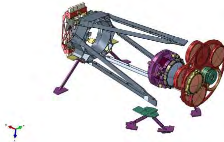
Figure 8-6 Wheels and lenses painted by material type
