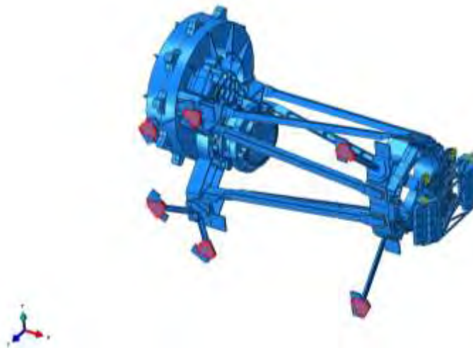
Figure 9-8 Bipods Thermal boundary condition surfaces
