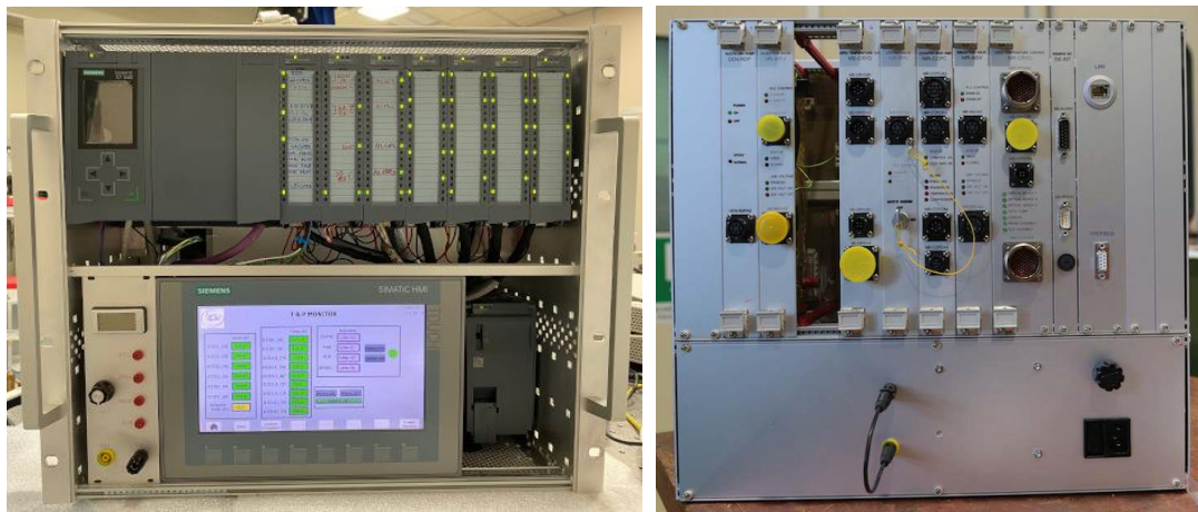
Figure 8. The Siemens sub-rack. Left: front view showing the PLC CPU, PDU, modules and touch panel. Right rear view showing the interface boards to the instrument. The board missing is the CFC one.
