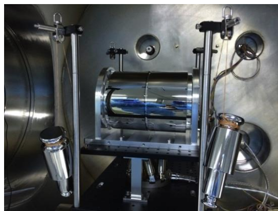
Figure 2. Left Panel: the effective area (single unit) of the current design of the eXTP SFA optics. On the right panel the very first prototype, successfully integrated at IPOE (Tongji University), is shown. The prototype has successfully passed vibration (5-6 g) and shock (5g) tests and its first performance testing session.
