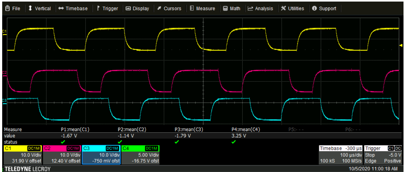
Figure 21 - Wipe vertical register (parallel phases)
