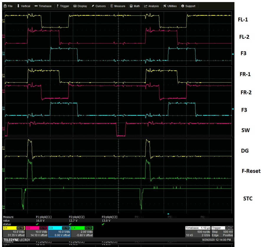
Figure 19 - Serial Right readout waveforms
