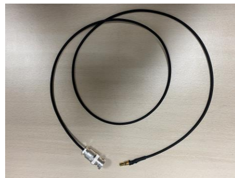
Figure 7 - Generator to preamplifier cable
