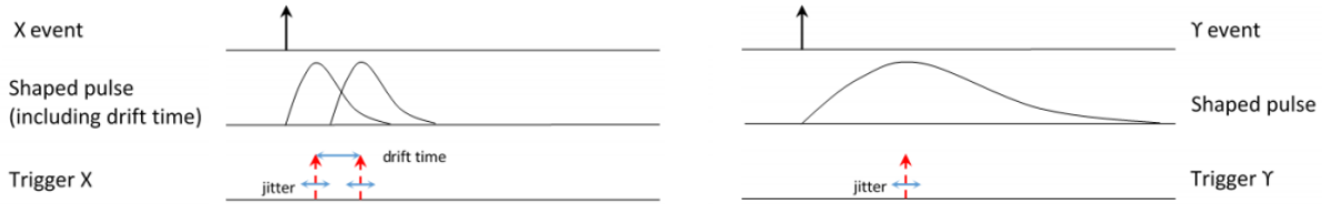
Figure 8. The time marking of the X and \gamma -events. Left : an X event is detected only in the top SDD but the time tag is affected by both the trigger jitter combined with the uncertainty due to the charge drift time due to the unknown interaction position within the SDD cell. Right : the time tag of a \gamma -event depends on the trigger jitter combined with a longer signal collection due to the fluorescence light component.
