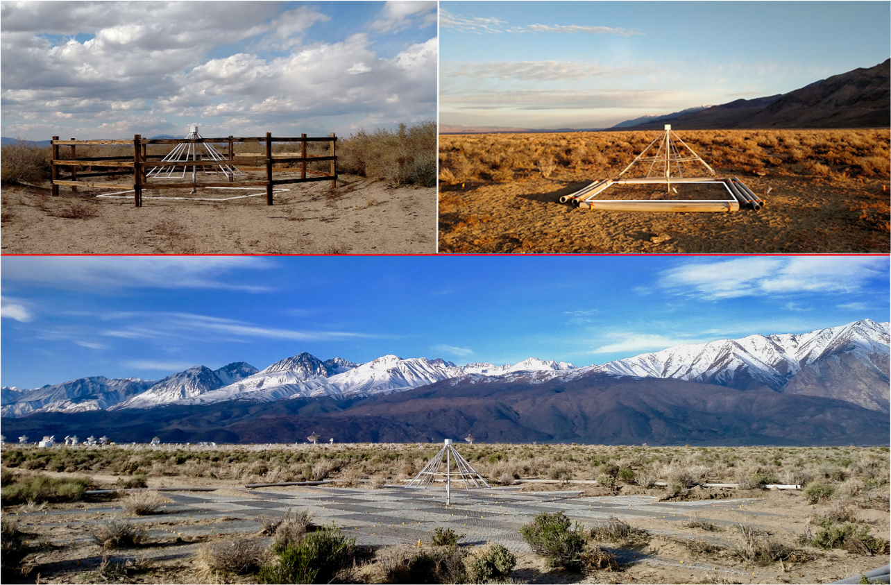
Figure 2. LEDA antenna 254, which sits in a slight depression surrounded by \sim 1 m-high woody vegetation (top left-hand panel), 252 prior to January 2019 (top right-hand panel), and 252 after (bottom) completion of the serrated ground screen in early 2019 April. Serrations that most strongly affect data were completed in February. The smaller ground screen (top figures) is 3 \times 3 m 2 (white boundary lines are intended to guide the eye) and flat to 10 cm peak to peak. The larger ground plane (bottom) is 20 \times 20 m 2 tip to tip and flat to 3 cm peak to peak. The antenna structure is aligned to within 1^\circ of true north and the antenna mast stands within 1^\circ of vertical. At antenna 252 (top right-hand panel), PVC pipes were used as a cattle guard in place of wood fencing because water absorbed from rainfall by the wood has the potential to affect the antenna gain response.
