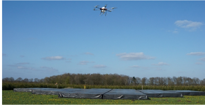
Fig. 1 The UAV after take-off is reaching the first waypoint to perform the required scan path over the LOFAR Eastern HBA array of the CS302 station. The array dimension is about 30 m.
