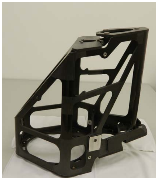
Fig. 3. CaSSIS CRFP structure
