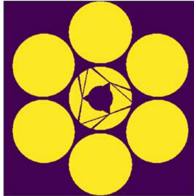
Figure 1-1 The true GMT pupil with center segment obscurations caused by the secondary mirror support structure shadows.
