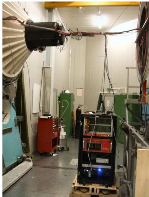
Figure 3. Left: Aqueye+ mounted at the T182 Copernicus telescope in Asiago. The MPD SPAD detectors are visible at the bottom. Right: Iqueye mounted at NTT. The rack at the base hosts the whole electronics system.
