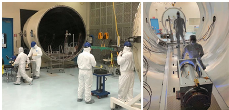
Fig. 14 (Left) Instrument chamber dome is removed for test-article integration into the chamber. The chamber is adjacent to an ISO7 (Class 10K) cleanroom. (Right) IXPE mirror module being installed inside the instrument chamber of the MSFC 100 m beamline facility. (Credit: NASA MSFC)
