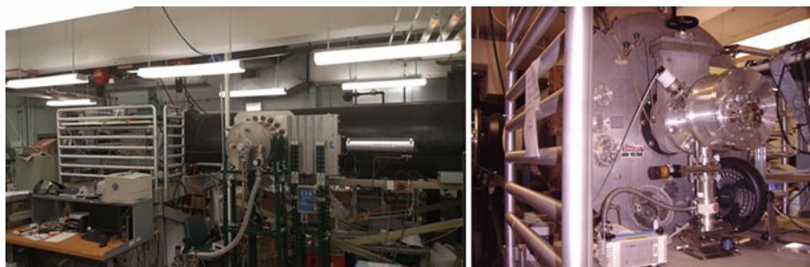
Fig. 19 Instrument end of PSU 47-m long X-ray calibration facility. (Left) Main cryopump mounted to the side of the beamline (black tube, 86-cm diameter). (Right) X-ray test camera mounted onto the vacuum door. Mirrors or entire instruments can be inserted into the 98-cm diameter experiment section. (Credit: PSU)
