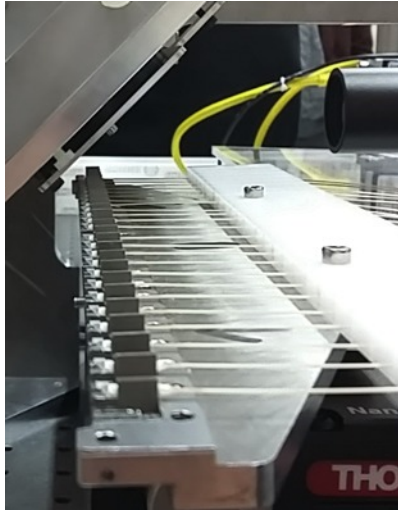
Figure 6: (left) The 24 fibres of the prototype bundle in place on the test setup for automatic measurements. (above) Closeup of the lensed top surface of one of the prisms showing the excellent centration achieved.
