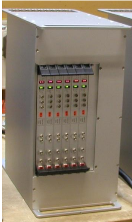
Figure 4. The NGC water-cooled housing
