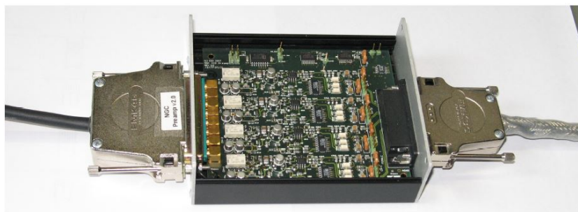
Figure 10. Detector Preamplifier (DPA).
