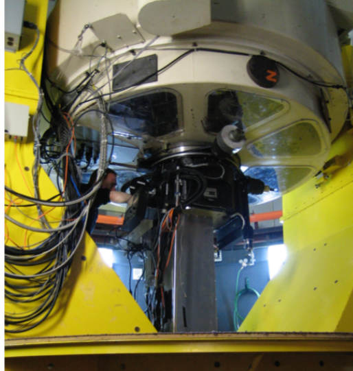
Figure 40: Generalised SCIDAR mounted at the focus of the Vatican Advanced Technological Telescope (VATT), telescope of 1.8 m located close to the LBT on the summit of Mt.Graham
