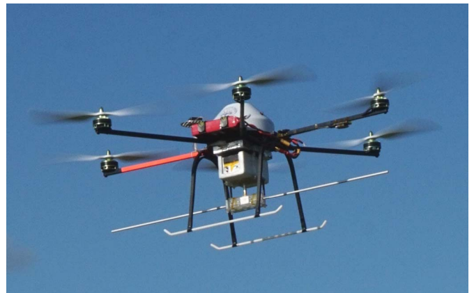
Fig. 1. Micro Unmanned Aerial Vehicle (UAV) equipped with RF synthesizer, dipole and differential GNSS receiver.
