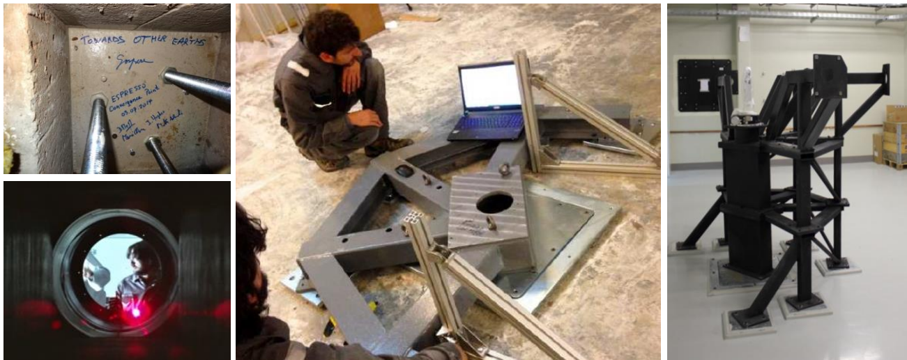
Figure 8: (top left) the central pin at the convergence point was the first hardware piece of ESPRESSO installed at Paranal, on July 3 rd , 2014; (bottom left) the laser tracker pointed in the Coudé Room of UT2; (center) balancer and plates during alignment before gluing; (right) FE structure mounted in the CCL.
