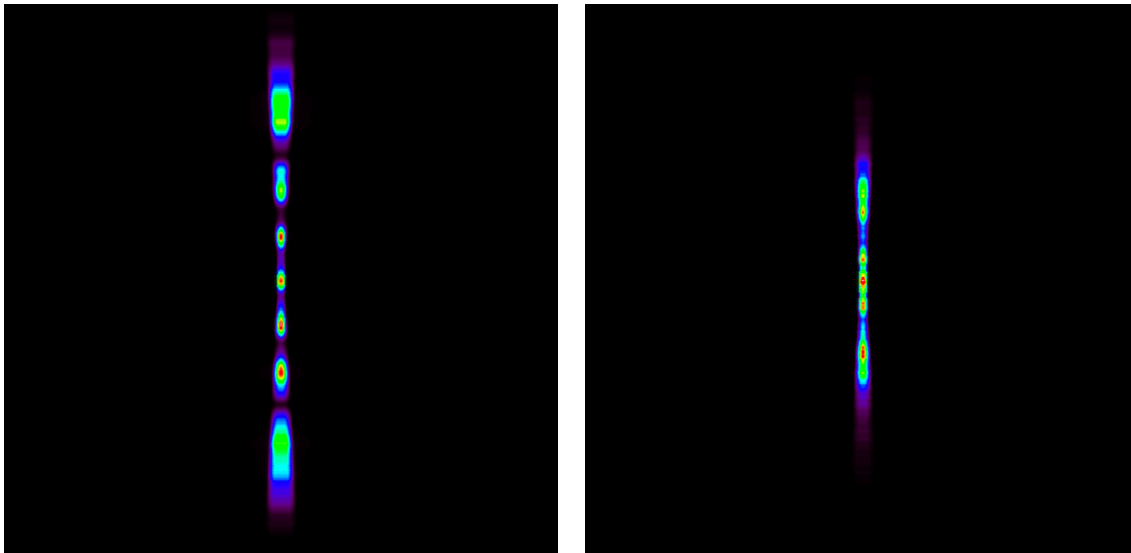
Figure 42: simulation at \lambda = 40 \text{ \AA} , 2 mm field, of the MM with a sinusoidal error along the plate length having (left) a period L and a constant 0.2 \text{ \mu m} amplitude on the primary stack. This multiple peak pattern corresponds to that of a sinusoidal grating with this period and amplitude. (right) the same, with randomized amplitudes, averages out the position of the peaks, so returning a much smoother PSF.
