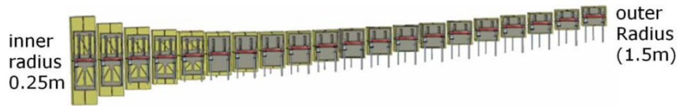
Figure 3: The Silicon Pore Optics (SPO) Mirror Modules (MM) are attached to the Mirror Structure (MS) via an isostatic mount, employing three dowel pins per MM. The principal surface of the telescope is a sphere with a radius f = 12 m, centred at the intersection of the optical axis with the focal plane.
