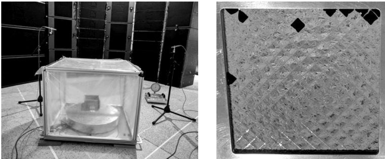
Figure 10. WFI OBF filter during acoustic tests at AGH University on April 2018. Filter wheel mock-up (left). Film failures at the test end (right). The metallic mesh stopped the propagation of the failures to the whole film.
