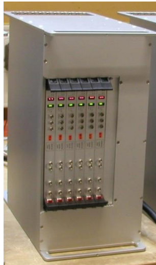
Figure 8 - The NGC water-cooling housing
