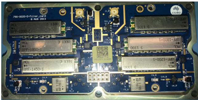
Figure 7. Photograph of the filter layer in the domino, referred to elsewhere as FILTER.
