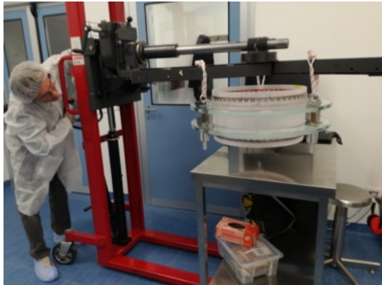
Figure 1: (A) The invar spoke wheel fixed on the Zeeko with new interfaces spacers to allow kinematic repositioning. (B) The system to dismount the shell from the Zeeko.
