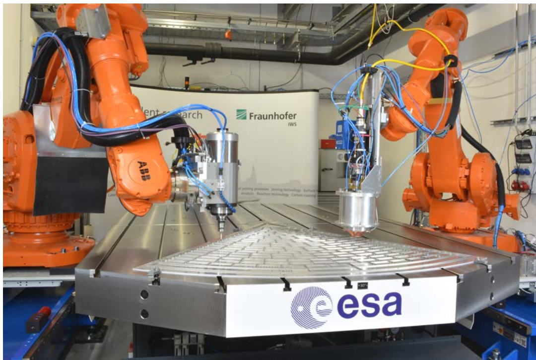
Figure 11: A novel titanium hybrid manufacturing facility is being set up to demonstrate the production of the monolithic titanium structure, which is baselined as the core of the ATHENA Mirror Assembly Module (MAM). This structure necessarily has a very complex geometry, since it has to accommodate the 678 MMs, and keep them accurately aligned from production over the launch sequence to the operation in space for the lifetime of the mission. Being a very large structure (2.5 to 3 m diameter, and about 300 mm high), it is difficult to manufacture with traditional (subtractive) machining. High precision industrial robots are used to position the tools over the high accuracy rotating platform. The right robot is used to add titanium material, using high power
