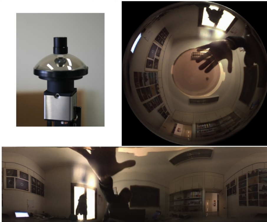
Fig. 6. The HH lens prototype (top left) and a “naked” recorded image (top right). Dewarped image (solely for the panoramic field) is shown in the bottom panel.
